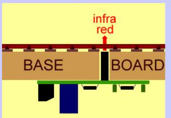
Where it is difficult to fit the detector due to baseboards
