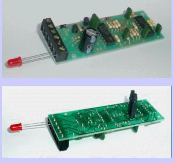
track wiring or the rolling stock. They are electrically separate from the track. This makes wiring simple. They work in both light and dark. The detectors are suitable for Z, N, HO, OO and O gauge.
